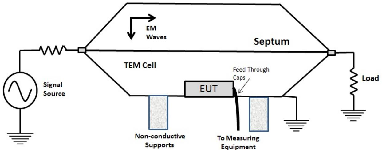
**Figure 5 - TEM Field for Parallel Plate Transmission Line**
